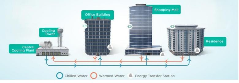
District Cooling (DC) produces cooling energy at a central location and then distributes it to multiple buildings through an underground network of insulated pipes. Chilled water is delivered to various buildings within a service area—such as offices, industries, and residential spaces. Each building's air conditioning system uses this chilled water to cool the air, making DC an efficient and sustainable cooling solution for large areas.
